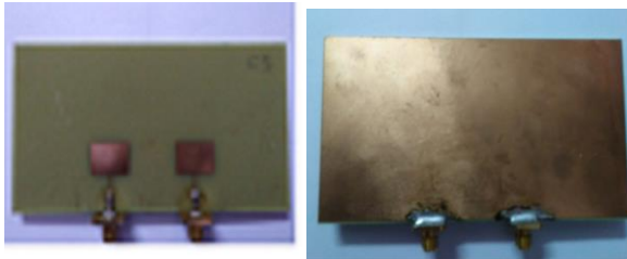
Figure 6. Photograph of setup of conventional microstrip antenna array for mutual coupling measurement (a) Front view (b) Back view
