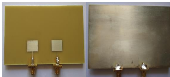
Figure 8. Photograph of setup of proposed microstrip antenna array for mutual coupling measurement. (a) Front view (b) Back view
