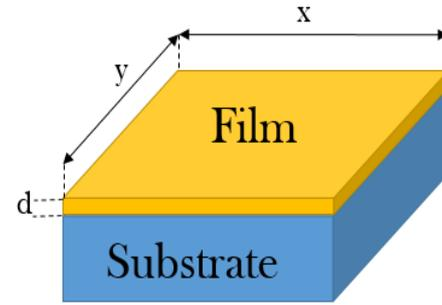
Figure 1. Schematic of ZnO thin-film deposited on glass substrate.
