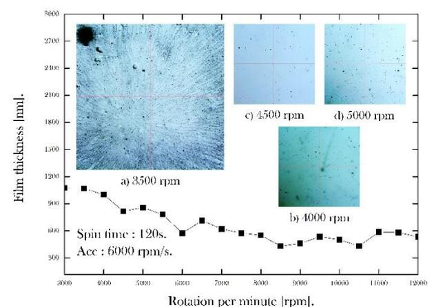
Figure 6. Evolution of film thickness according to rpm.
