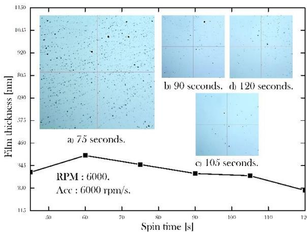
Figure 5. Evolution of film thickness according to spin time.
