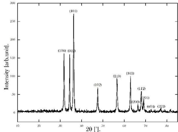
Figure 2. Diffractogram of ZnO annealed at 400°C for 2h.
