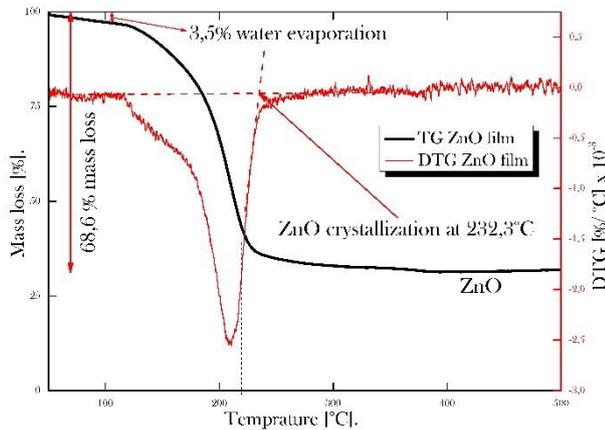
Figure 3. TG and DTG thermograms of ZnO.
