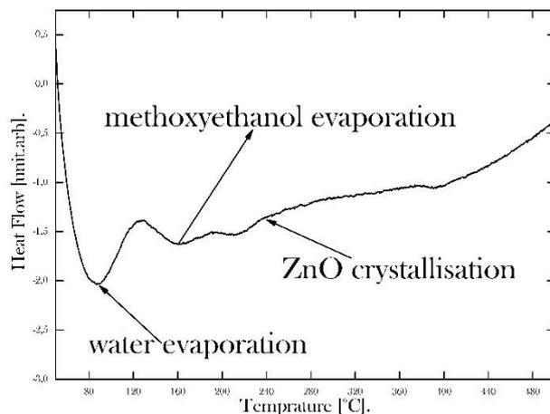
Figure 4. DSC thermogram of ZnO.
