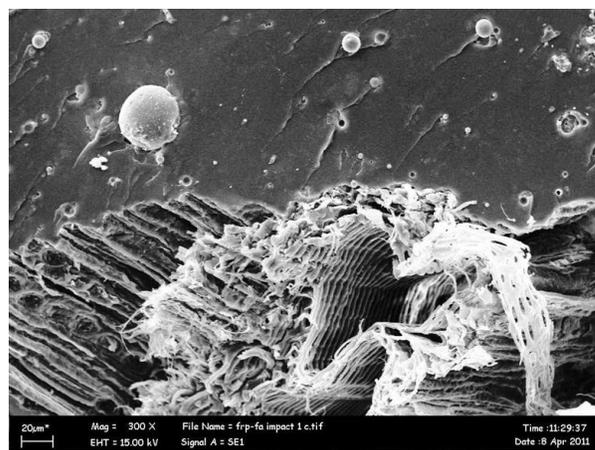
Figure 7. Fractography of fiber-ash-polyester composite
