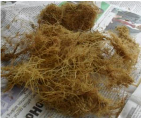
Figure 1. As-received oil palm fibers
