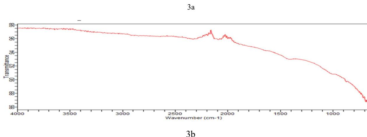
Figure 3. FTIR spectra for *Gmelina aborea* (3a) and inhibited corrosion product on aluminium surface (3b)
