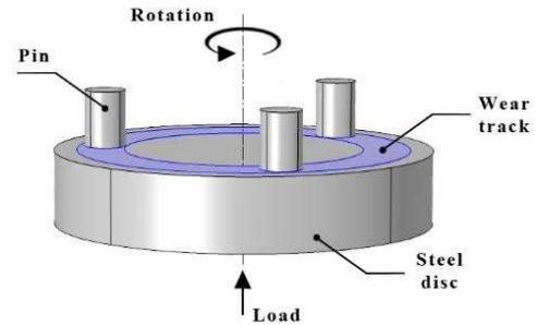
Figure 2. Schematic of pin-on-disc configuration
