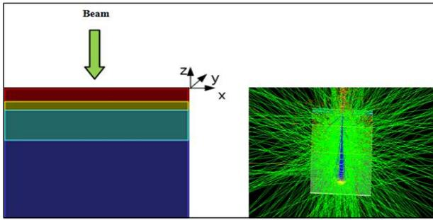
Figure 6. Schematic representation of the heterogeneous configuration used: The different materials are represented by different colors; in red: soft tissues, in yellow: cortical bone, in blue: lung, and in dark blue: water, (left). Screen shot of the interactions of proton beam in the phantom (right).
