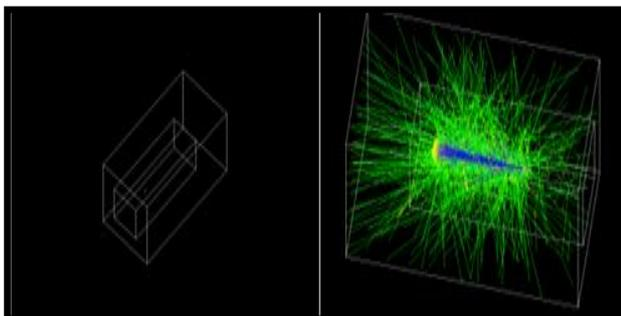
Figure 4. (left) Mother volume containing water phantom, (right) interaction of proton beam in water phantom
