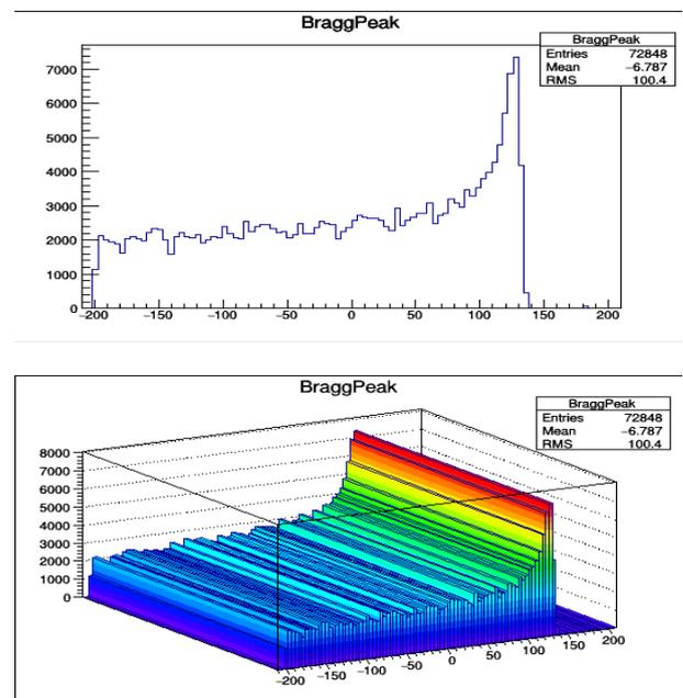
Figure 5. (a)Depth-dose profiles (Bragg Peak) generated from the interaction of scenario 1, the depth of deposit dose is in 150 mm in water with mean energy of 79 MeV, (b) 3D projection of the Bragg Peak.
