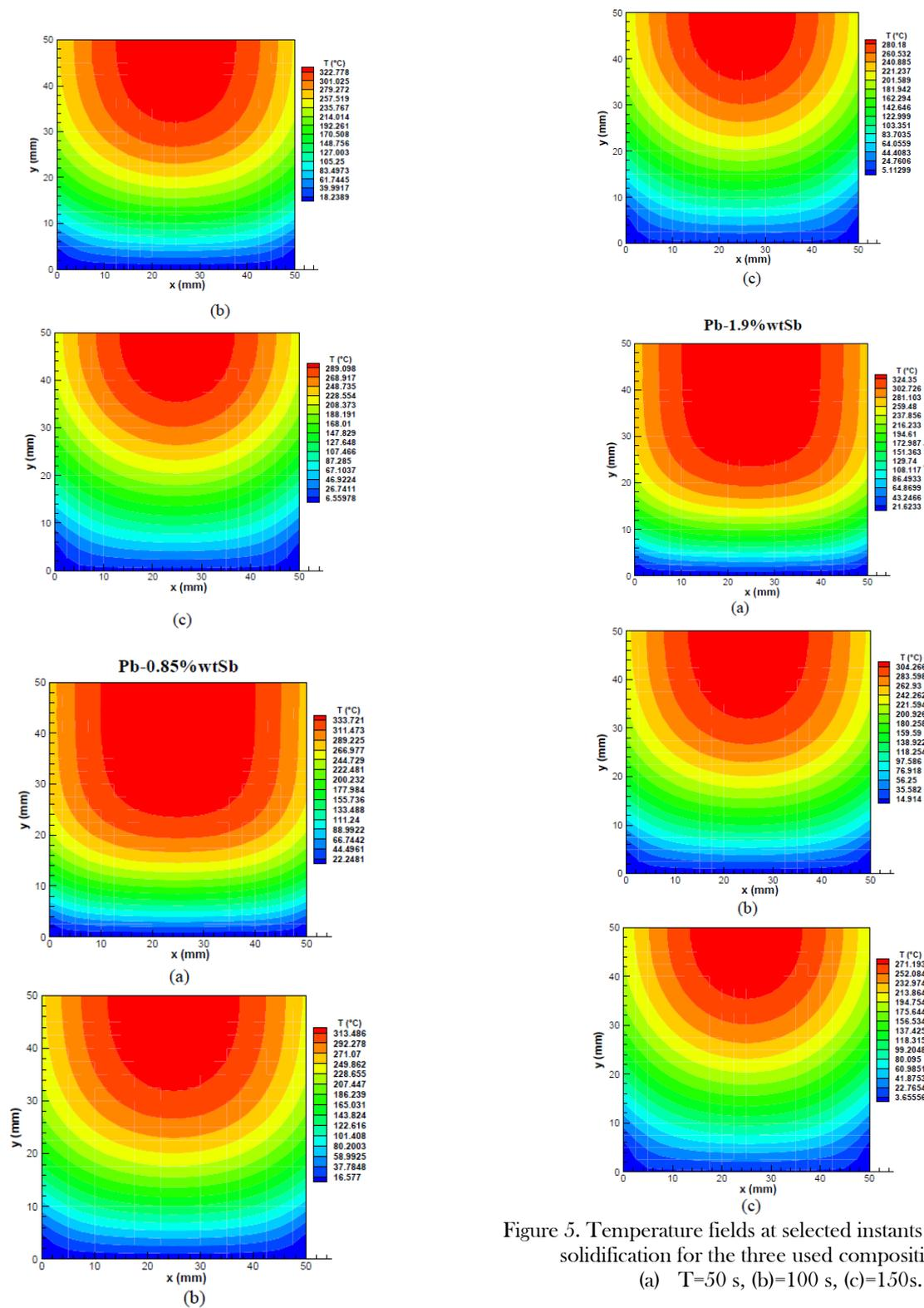
Figure 5. Temperature fields at selected instants during the solidification for the three used compositions: (a) T=50 s, (b)=100 s, (c)=150s.
