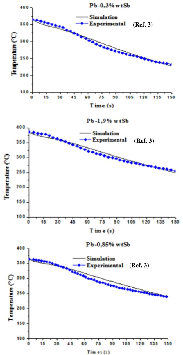
Figure 4. Variation of the temperature as a function of cooling time for the Pb-Sb alloy.
