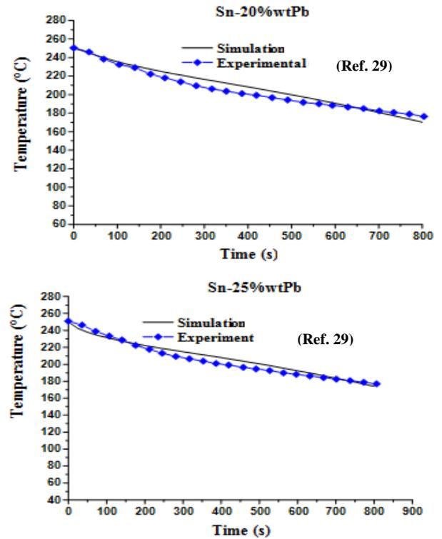
Figure 2. Variation of the temperature as a function of cooling time for the Sn-Pb alloy.
