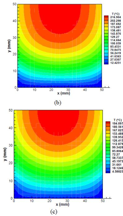
Figure 3. Temperature fields at selected instants during the solidification for the four used compositions: (a)  $T=50$  s, (b)=100 s, (c)=150s.
