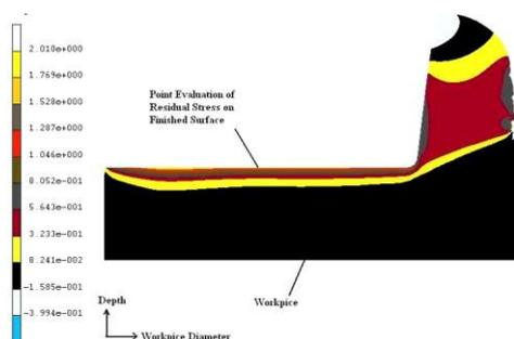
Figure 3. Surface and subsurface residual strain profile in the cutting (circumferential) direction [48].
